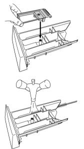
7. Use a brush to clean the entire rinsing-in part of the washing machine, especially the nozzles on the top side of the rinsing-in chamber.
